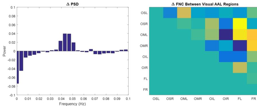
**Figure 3: Representative examples of the two types features used as input to the machine learning algorithms. (left)  $\Delta PSD$ , the changes in power/frequency and (right) Seasonal  $\Delta FNC$  matrix (upper triangular portion).**
