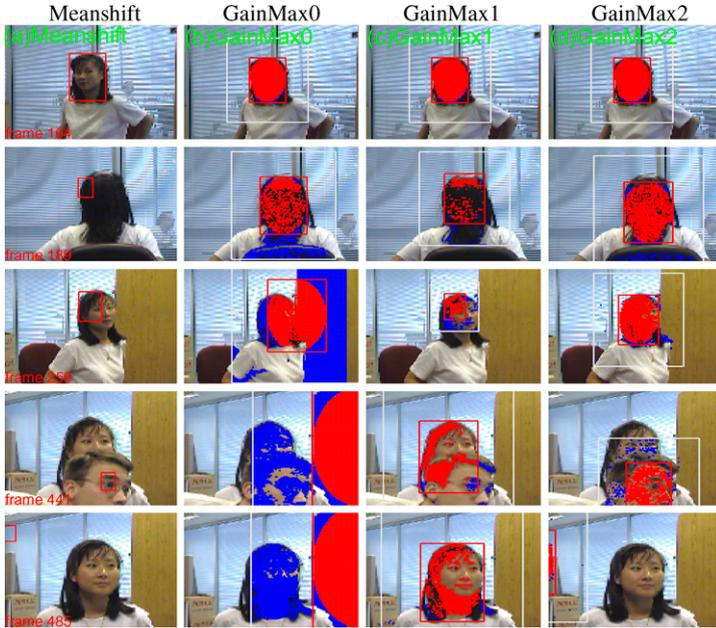
**Fig. 19.8** GainMax trackers using gradient ascent information gain maximization can handle distraction and occlusions well. For the mean-shift tracker (column 1), the red box is the tracking result; for GainMax trackers 0–2 (columns 2–4), red indicates pixels correctly labeled in the ellipsoid as target (true positive), blue indicate false positive pixels outside of the target ellipsoid
